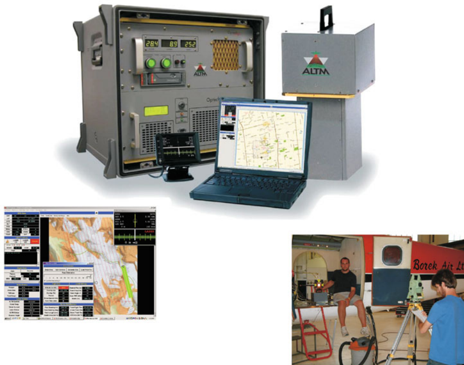
LIDAR in Glaciology, Figure 1 Top : Schematic of the measurement and reference framework for airborne lidar mapping; Middle : Typical ALTM system components including, clockwise from top left : console containing the control module, data storage, IMU and GNSS system interface and laser power supply; laser/mirror assembly; notebook computer/operator interface; pilot display; Bottom : Surveying mechanical offsets for an installation in a de Havilland Canada Twin Otter (System photograph courtesy Optech Inc., Toronto Canada; photograph of mechanical offset measurement courtesy Chris Hopkinson and the Canadian Consortium for Lidar Environmental Applications Research, C-CLEAR).
